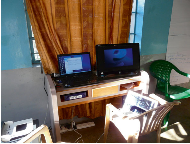
Fig. 8.3 A simple two-screen workstation consisting of a laptop computer connected to a single 22 in. 1080p external monitor. The larger monitor is used for image display and the smaller for text
