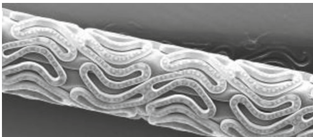
Fig. 19.17 Abluminal coating of Paclitaxel/D,L-PLA dots on JacTax™ DES [40]
