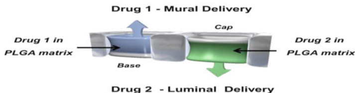
Fig. 19.14 Schematic of reservoir-based dual drug-eluting Stent
