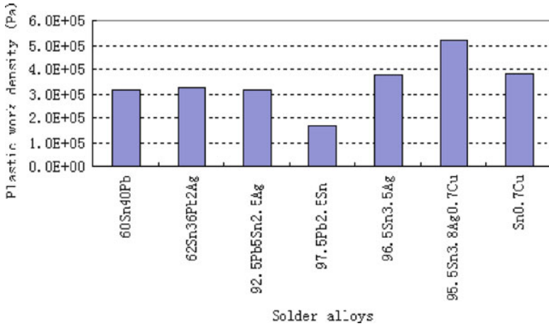
Fig. 5.17 Plastic work density comparisons for different solder joints
