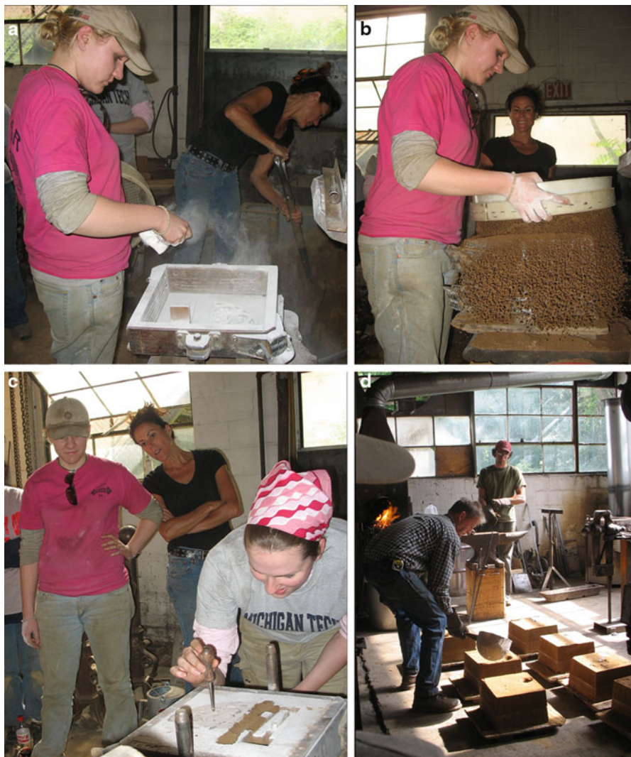
Fig. 8.2 Michigan Tech industrial archaeology students, both undergraduate and graduate, draw upon experiential learning activities, such as making these molds for casting aluminum at Super Square Foundry in 2006: (a) Lindsay Kiefer coats a wooden pattern and mold with parting compound as Amy Lahey prepares molding sand; (b) Lindsay sifts sand into the mold before packing it around the pattern; (c) Stephanie Atwood removes the pattern from the packed mold; (d) Dean Andersen pours metal into the molds (photos courtesy of Michigan Technological University)
