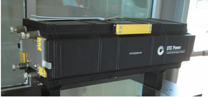
Fig. 9.37 UTC power's S300 automotive fuel cell stack
