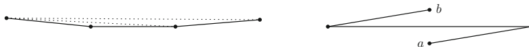
Fig. 16 A path with unit length edges, which requires an edge of length 3 - \varepsilon for 2-edge-connectivity augmentation ( left ). A path between a and b , where the stretch factor is large but cannot be improved with additional edges ( right )
