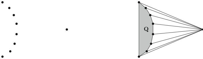
Fig. 9 A set S of n = 9 points with a triangular convex hull (left). A maximal plane graph on top of S will be a triangulation T with 3n - 6 edges. However, the edges shown on the right must appear in every triangulation of S , and they only differ in the edges that triangulate the gray region Q . Therefore, T will have at least two vertices of degree 3, and at least one with degree n - 1
