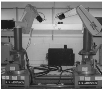
Fig. 8.3 Experiment testbed of two PUMA 560 arms: Mounted on the wrist of each arm is a six-degree freedom force/torque sensor.
