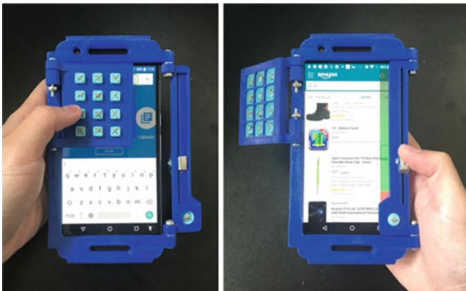
Fig. 36.5 Interactiles allows people with visual impairments to interact with mobile touchscreen phones using physical attachments, including a number pad (left) and a multipurpose physical scrollbar (right)
