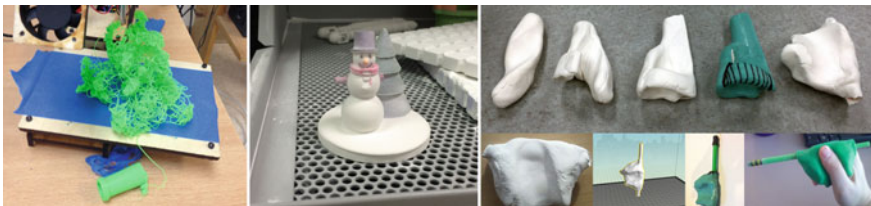
Fig. 38.2 Common printer failure where the model came loose from the print bed resulting in wasted filament and time (left). Delicate and full-color 3D print made at a school for the blind (middle). Design exploration (in clay) with therapists in a school setting to create a custom stylus grip for a student (right). All photos were taken by Erin Buehler
