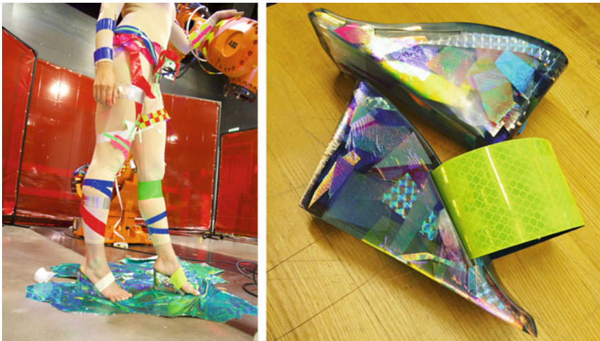
Fig. 4 Left: Computer Enhanced Footwear Prototype 3 worn by Dancer Elizabeth Bressler. Right: CEF P3 ; showing outcomes of embedded mylar in every 100 slices of the 3d print. Pier 9, Autodesk, San Francisco, 2016. Photos by Alexandra Murray-Leslie
