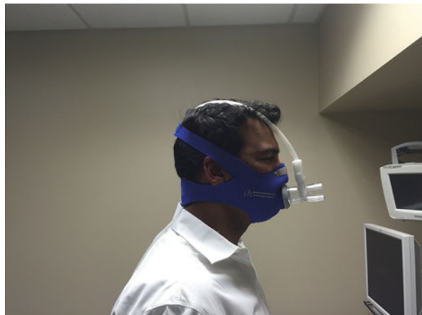
Fig. 5.1 Air-sealed face mask with tubing connected to gas analyzer, used to determine gas flow and values during metabolic testing
