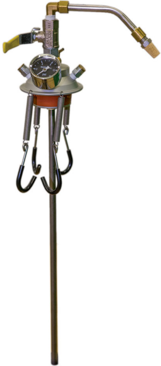
Fig. 11.1 Withdrawal device for dewars of 20 l and over. (Brymill™): Conveniently fills multiple delivery units at a time. Affixes to the top of the dewar (i.e., is not removed after each use), has a simple on/off switch, and works like a faucet. Includes a filter that helps clean the LN before it is withdrawn
