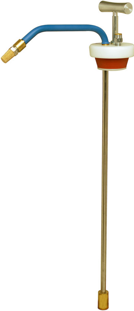
Fig. 11.2 Withdrawal tube for dewars of 5–20 l. (Brymill™): Simple and efficient way to extract LN from a storage dewar. Fills one to a few delivery units at a time. The tube is removed from the dewar after each use. Offers quick pressurization. Includes a filter that helps clean the LN before it is withdrawn
