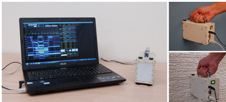
Fig. 14.78 “Wood wall viewer” using FMCW radar system
