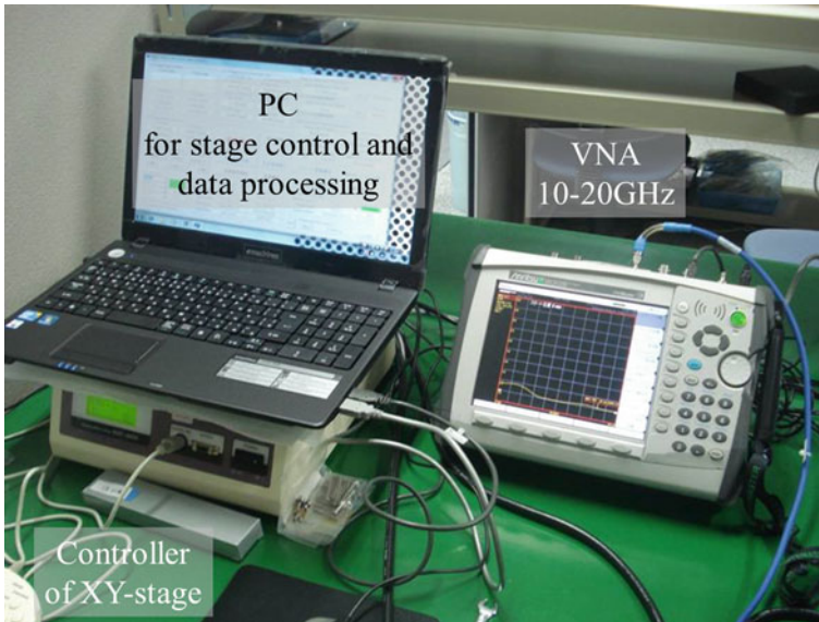
Fig. 14.71 Experimental setup of FMCW radar system to get time-domain signal
