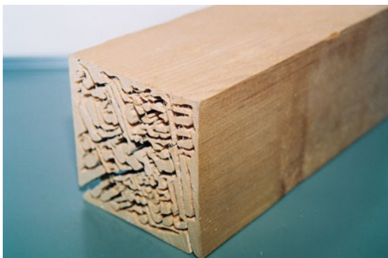
Fig. 14.53 Wood attacked by termites
