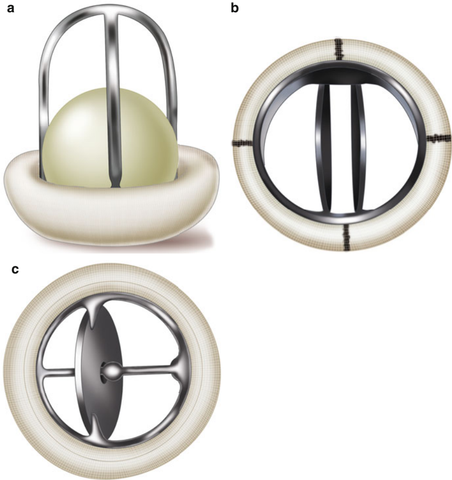
Fig. 21.3 Common mechanical heart valves: (a) Ball in cage design. (b) Bileaflet tilting disc. (c) Tilting disc
