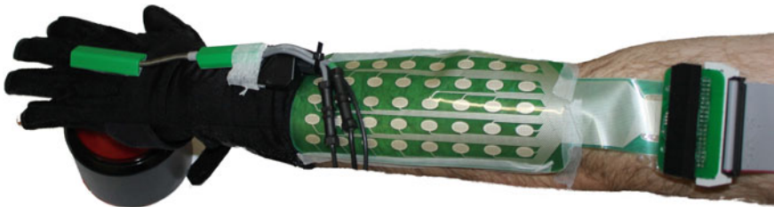
Fig. 6.1 Electrode array with data glove and electrogoniometer used for stimulating and tracking hand and wrist movement
