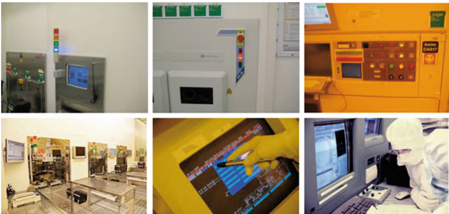
Fig. 12.2 Equipment interfaces at the factory: the first row shows the heterogeneous signal lights of different equipment (depending on the manufacturer); the second row shows the heterogeneous interfaces, which can be used to control equipment
