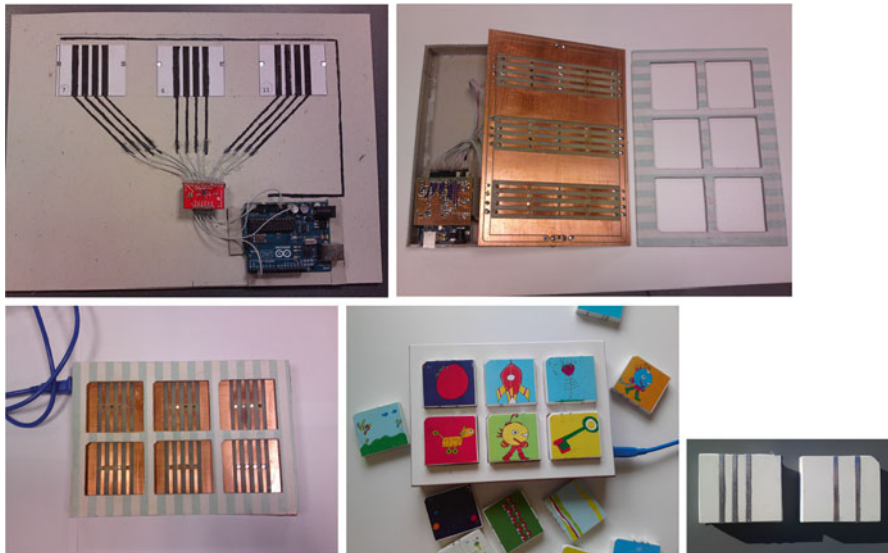
Fig. 12.3 Proof of concept ( top left ); first functional electronic prototype ( bottom left ); prototype with blocks ( bottom centre ) and backside of two blocks ( bottom right )
