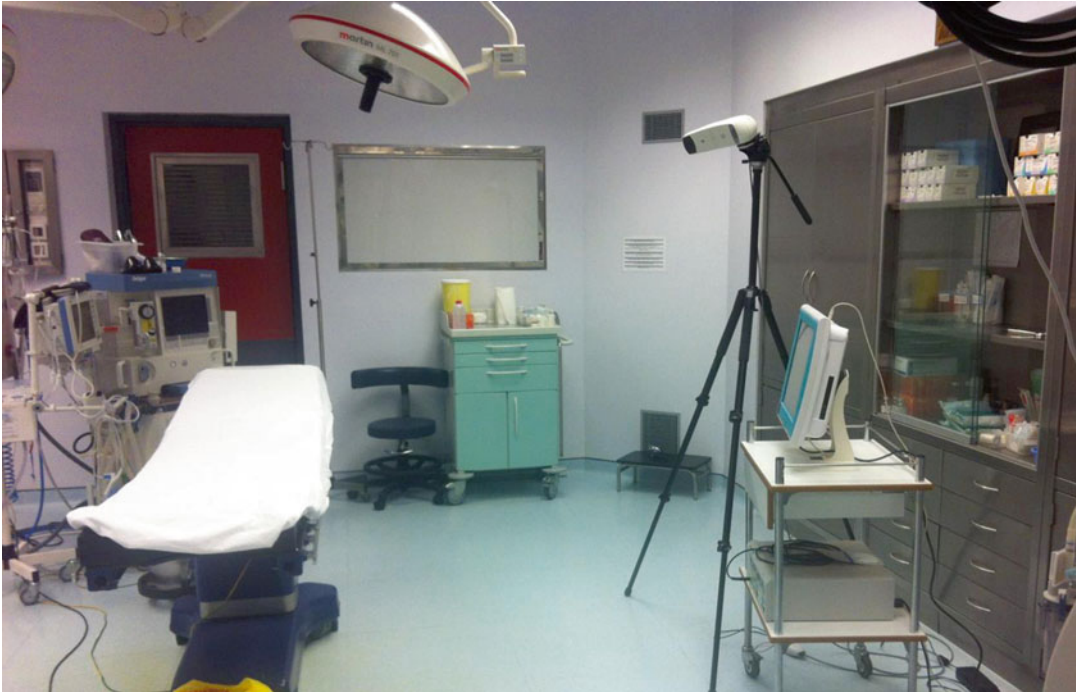
Fig. 25.1 The detector device used to monitor relevant object in the operating field, collecting real time data relating to their location and orientation is shown. It detects the joint and the instruments position and need to
