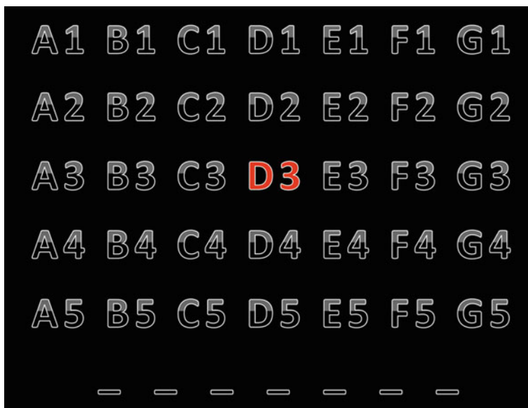
Fig. 3.3 A basic P300 composer interface. In the above image, the note-letter D3 is flashing. If the user is attending to D3 at that moment, there should be an increase in amplitude detectable in the averaged signal after each complete trial run. Note that although this display shows 5 octaves in the key of C, there are no restrictions in terms of which note-pitch values and controls can be represented
