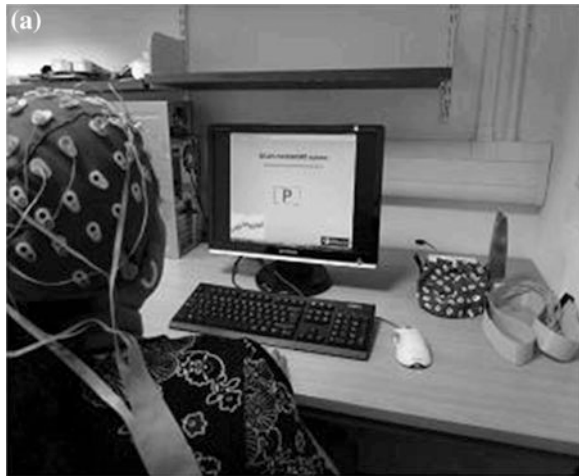
Fig. 2.4 BCI system a a user using BCI and b 10–20 electrode configuration
