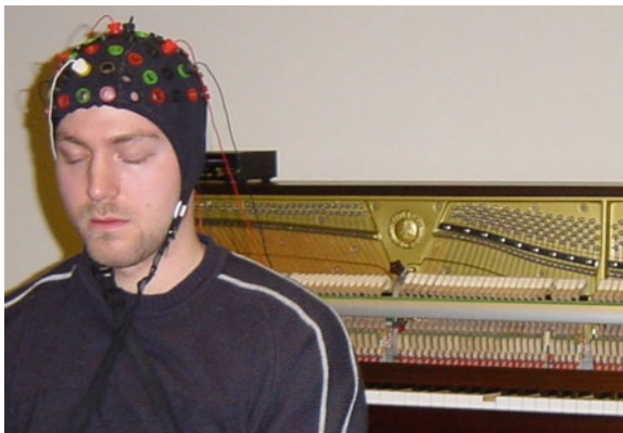
Fig. 1.1 With BCMI-Piano one can play music generated on the fly on a MIDI-enabled acoustic piano with brain signals. No hands needed
