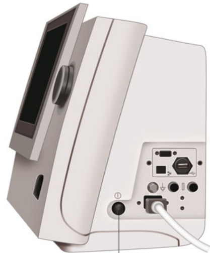
Power switch on right side of impella controller
