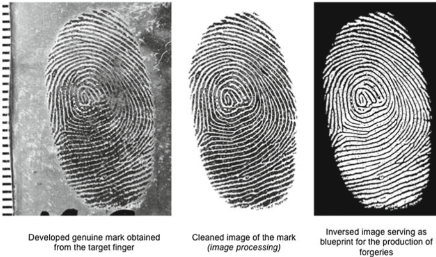
Fig. 2.7 Preparation of the blueprint (tonally reversed with white ridges black furrows ) that will serve for the preparation of the forged marks without the cooperation of the donor
