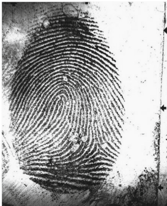
Fig. 2.11 Forged marks developed with aluminium powder by Morisod [32]. The mark originates from a genuine mark of sebaceous residue left on glass and transferred onto another piece of glass using a gelatine lifter (note the marks left by the edges of the lifter and the air bubbles left during the transfer process)
