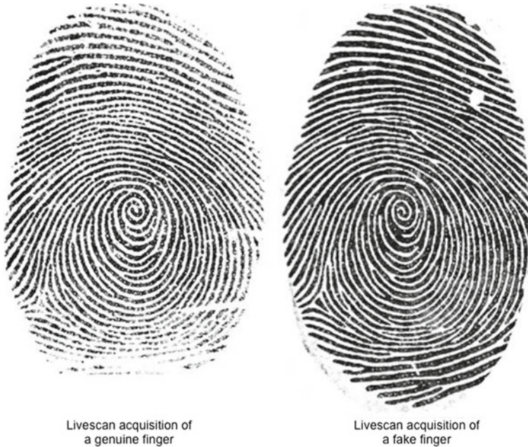
Fig. 2.8 Comparison between a genuine and a forged finger acquired on an optical livescan device. The forgery has been prepared without the cooperation of the donor starting with a mark detected optically on a glass surface and a latex cast (Gédéo, France)
