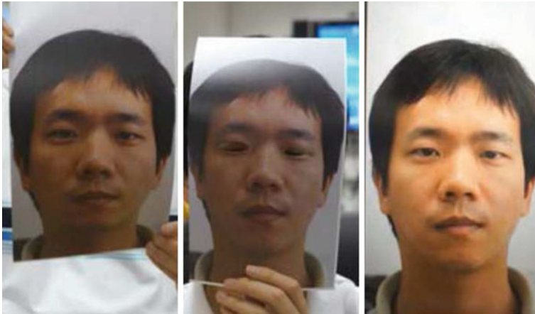
Fig. A.12 Samples showing the three types of attacks present in the CASIA-FASD. From left to right warped photo, cut photo and video attacks, from [13]
