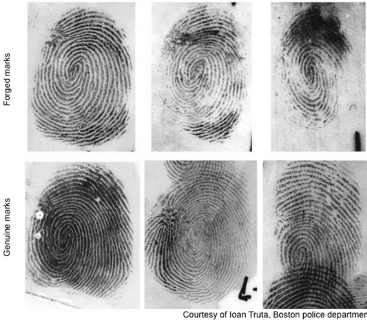
Fig. 2.5 Genuine and forged marks deposited by Ioan Truta (Boston police department) on white backing cards and detected with black magnetic powder . The forgery has been prepared using a double casting technique with the cooperation of the donor, the first mould in putty and second mould with AccuTrans
