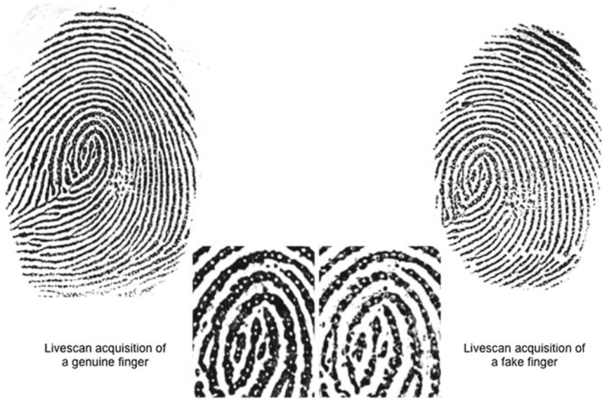
Fig. 2.6 Comparison between a genuine and a forged finger acquired on an optical livescan device. The forgery has been prepared using a double casting technique with the cooperation of the donor, the first mould is made in a thermoplastic (UtilePlast, Pascal Rosier, France), the second is a silicon molding paste (Siligum, Gédéo, France)
