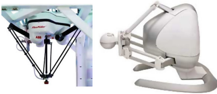
Fig. 8.8 Left FLEX PICKER for pick-and-place tasks (source ABB); right the FALCON as a 3-DoF haptic device (source Novint Technologies Inc.)
