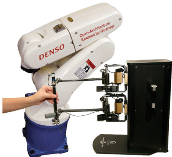
Fig. 1.8 Versatile teleoperation by Quanser : HD 2 haptic interface with 7 DoF of haptic feedback and DENSO OPEN ARCHITECTURE robot with 6 DoF. Image courtesy of Quanser , Markham, Ontario, CA
