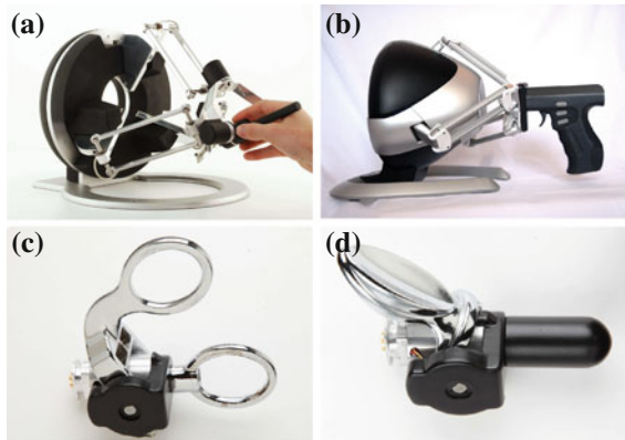
Fig. 2.29 Realizations of tool-mediated contact in commercial haptic interfaces. a OMEGA.6 with a stylus interface ( Force Dimension , Nyon, Switzerland), b FALCON with a pistol-like grip for gaming applications ( Novint , Rockville Centre, NY, USA), and c and d pinch and scissor grip interfaces for the PHANTOM PREMIUM ( 3D Systems Geomagic Solutions , Rock Hill, SC, USA). Images used with permission
