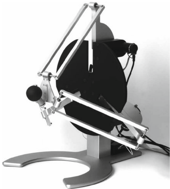
Fig. 6.4 Example of a parallel kinematic closed-loop impedance controlled system (delta3, ForceDimension ). Image courtesy of ForceDimension , Nyon, Switzerland, used with permission
