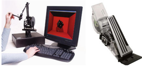
Fig. 2.28 Two haptic interfaces, PHANTOM PREMIUM 1.5 ( 3D Systems Geomagic Solutions , Rock Hill, SC, USA) and ACCELERATOR FORCE FEEDBACK PEDAL (AFFP, Continental Automotive , Hannover, Germany). Images used with permission
