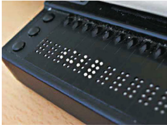
Fig. 6.6 Example of an open-loop admittance controlled system being a Braille row. Image courtesy of Ralf Roletschek, used with permission
