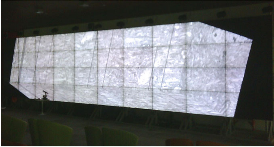
Fig. 29.2 A high-resolution electron microscopy (EM) volume of brain tissue, rendered on a large display wall consisting of 10 \times 4 individual LCD displays. Each screen has a resolution of 1,366 \times 768 , leading to a total display resolution of 13,660 \times 3,072
