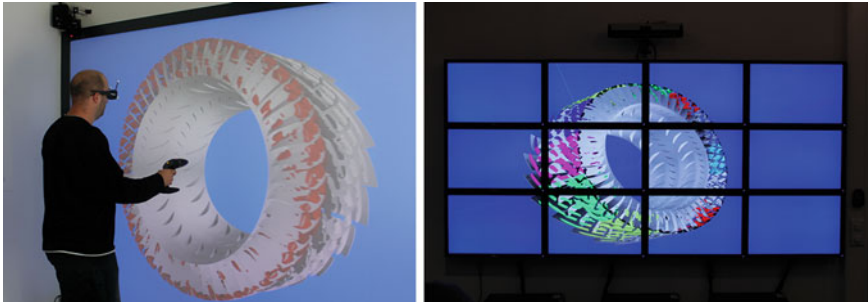
Fig. 31.11 Hybrid rendering allows interactive analysis of complex geometry like the depicted compressor tera-byte dataset on a powerwall ( left ) and on a display wall ( right ). The surface geometry is rendered locally at high frame rates whereas isosurfaces are rendered remotely
