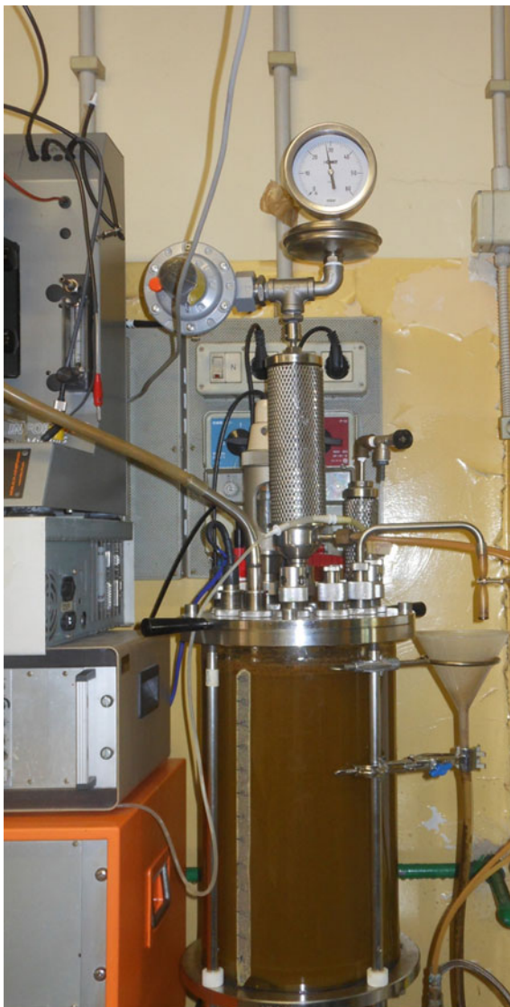
Fig. 8.2 Chemap-Fermenter of 14 L used for the batch tests
