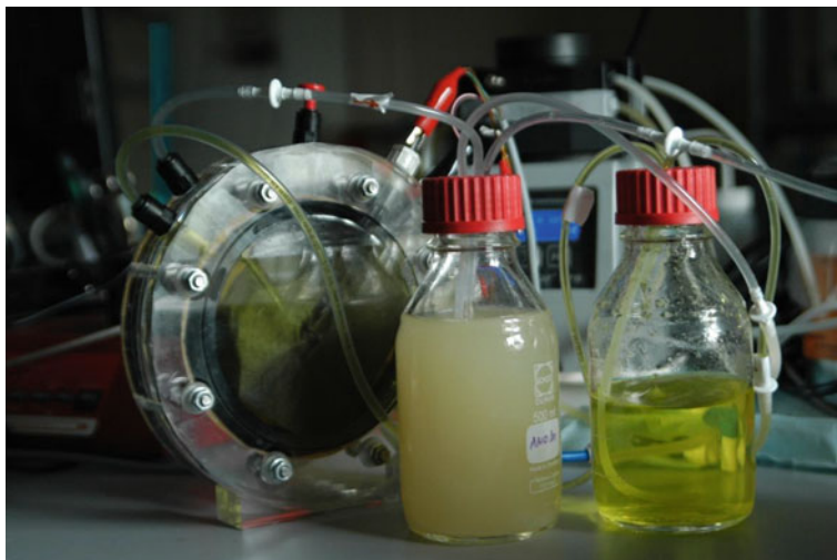
Fig. 7.7 MFC design used to conduct tests for continuous generation of electricity
