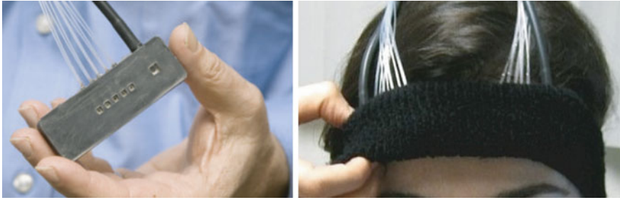
Fig. 6.1 Left We display one example of an fNIRS probe with four light sources and one detector. Right A researcher uses a headband to secure two probes to a user's forehead
