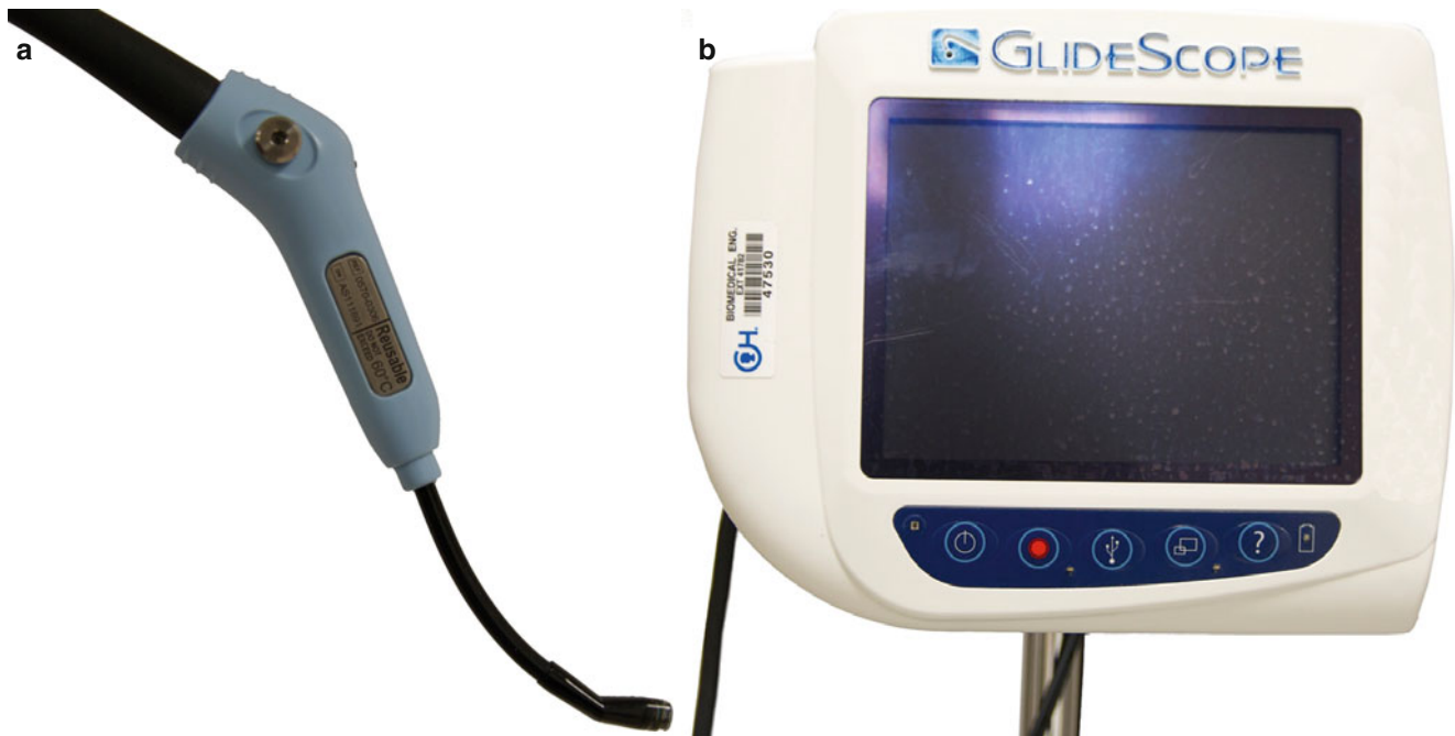
Fig. 28.3 (a) Glidescope Cobalt. A reusable video baton that delivers an image to a portable monitor. The video baton inserts into different sized curved plastic disposable laryngoscopy blades. Various sizes of
