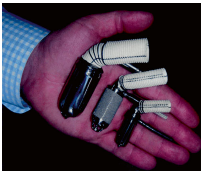
Fig. 26.9 The adult, child, and infant Jarvik 2000® devices. The infant model is still at the conceptual prototype stage of development
