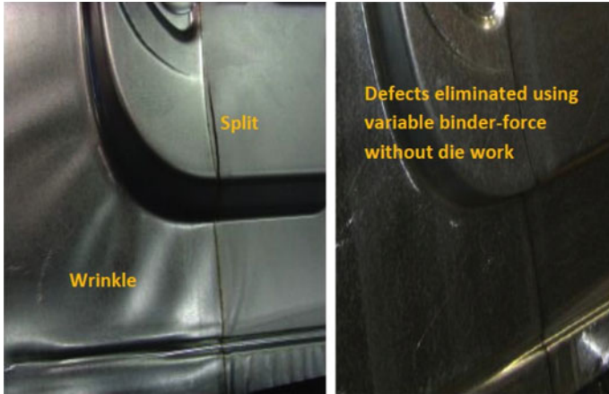
Fig. 4.8 Forming defects eliminated using variable binder force
