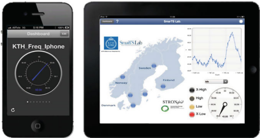
Fig. 13 iPhone and iPad PMU data visualization Apps powered by Statnett’s SDK PRL interface
