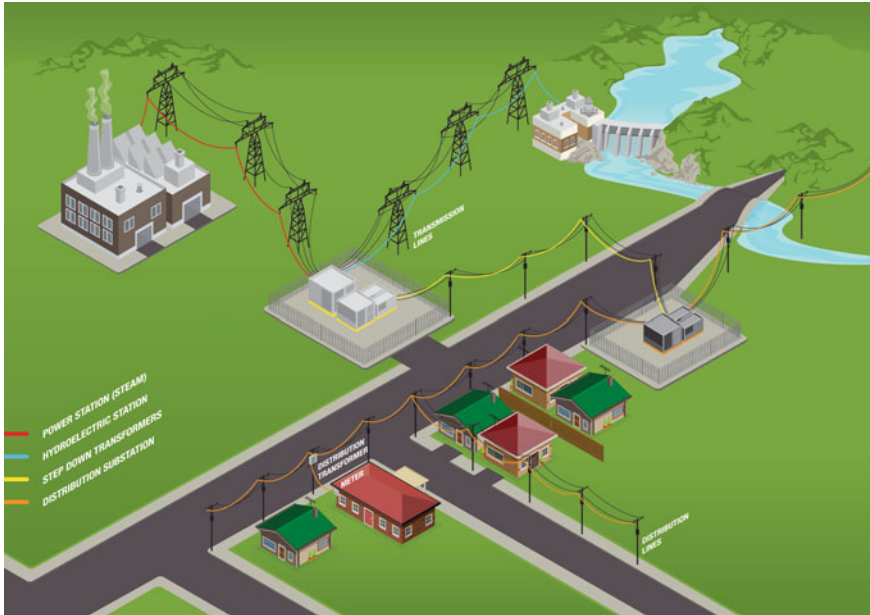
Fig. 1 A simplified view of electricity generation and transfer [10]
