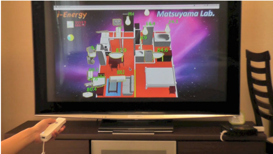
Fig. 5 Real-time visualization of individual appliance power consumption: Every 0.5 s, the consumed power is displayed on top of each appliance icon. By clicking an appliance icon, we can monitor its power consumption profile as well as control its supplied power. The overall power consumption pattern in the apartment room can be monitored to analyze which appliances consume how many watts
