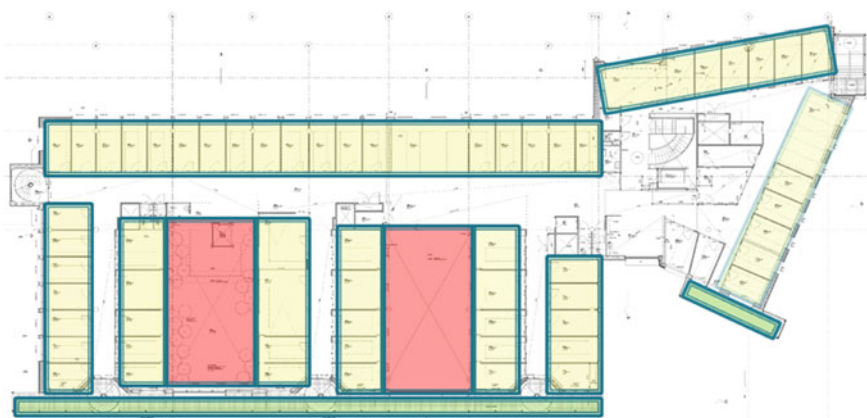
Fig. 10 Grouping office rooms (shown with yellow colour) around closed inner courtyards (with red) increases the depth of the building and results in improved compactness
