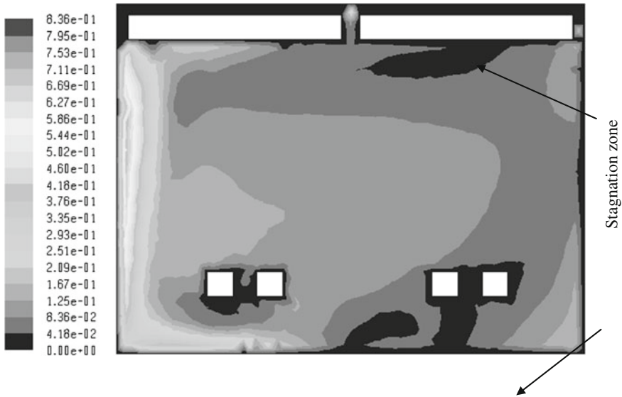
Fig. 14 Contours of velocity magnitude (m/s) at H_{CC} of 3 m, Z-Y, X = 3 m
