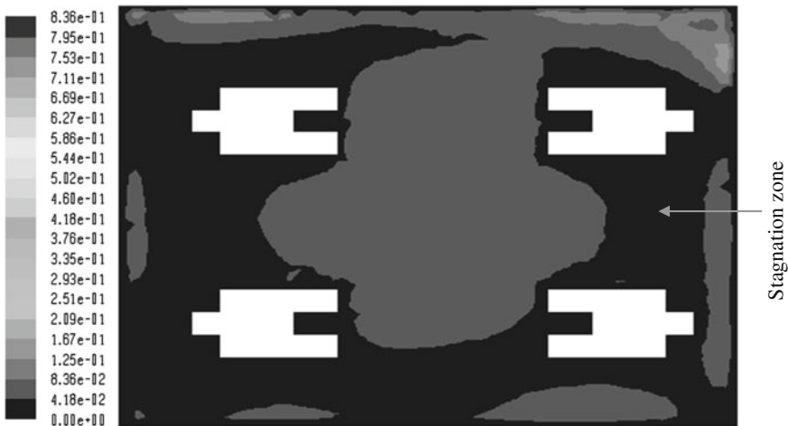
Fig. 17 Contours of velocity magnitude (m/s) at H_{CC} of 2 m X-Z, Y = 0.6 m
