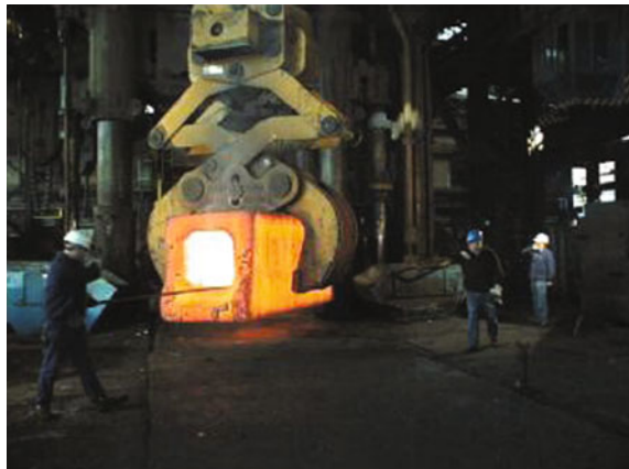
Fig. 4.28 Forging part of the inner leg curved section of a TF coil case as a hollow tube. Courtesy of ITER Organization
