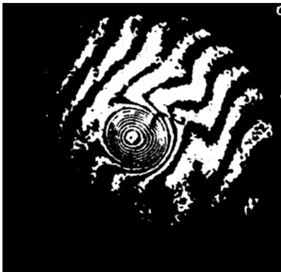
Fig. 11.59 Fringe pattern of a theta pinch plasma, taken with a Mach-Zehnder interferometer (courtesy of Los Alamos National Laboratory)
