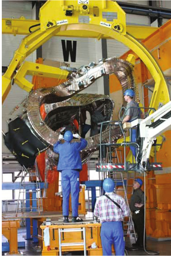
Fig. 4.45 A modular coil is strung onto a segment of the plasma vessel. (Courtesy of Lutz Wegener, Max-Planck Institut für Plasmaforschung, Greifswald, Germany)
