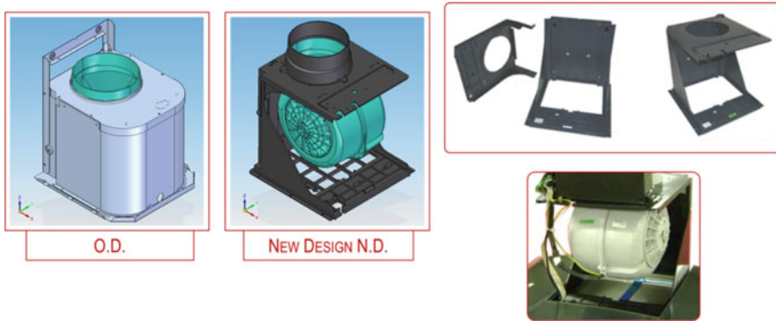
Fig. 5 Solution adopted in the new design configuration of blower system support and comparison with the original solution
