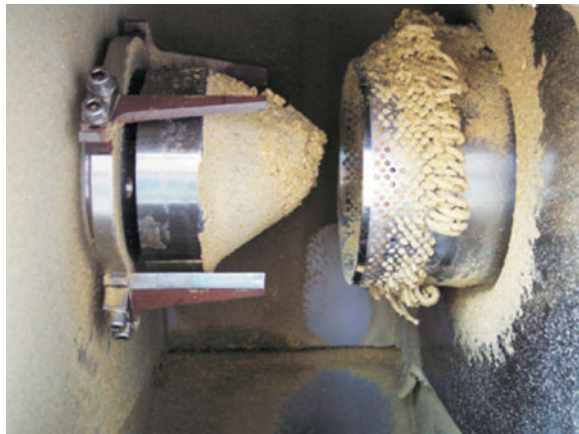
Fig. 3 Crown expander after shutdown
