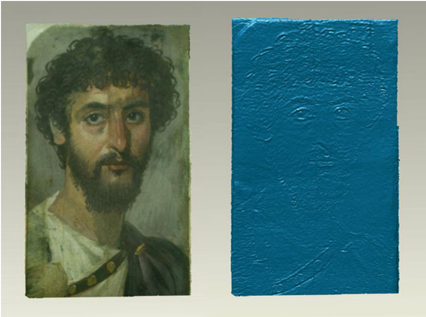
Fig. 2.3 Photograph and colour-stripped, artificially lit 3D model derived from laser scanning data. The 3D data reveal both the depth of paint in the image and the indentations relating to the initial sketching of the image prior to painting
