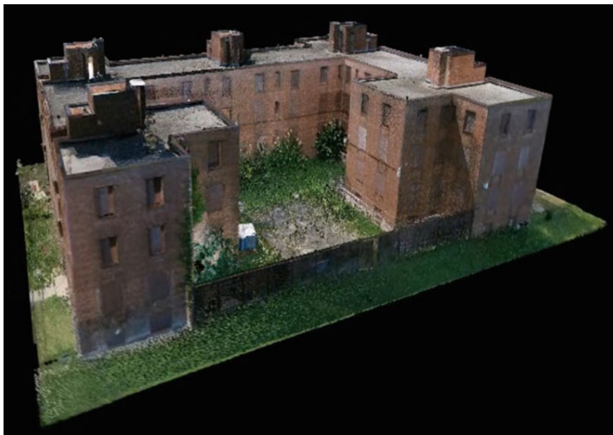
Fig. 2.7 Point-cloud data of the exterior of the National Public Housing Museum
