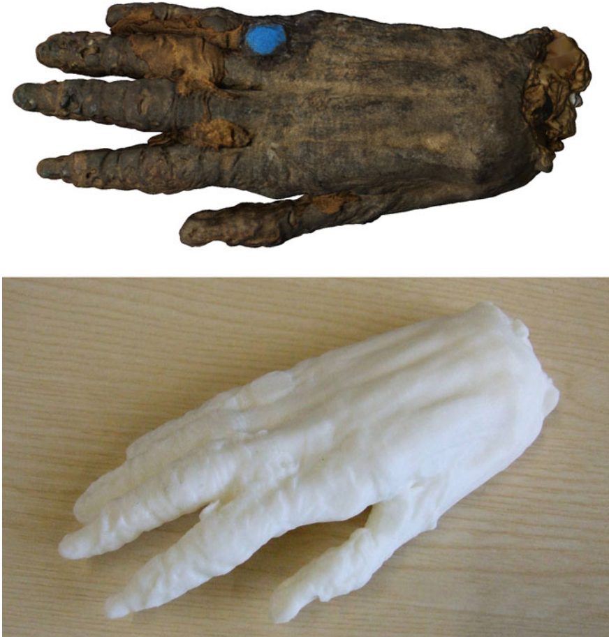
Fig. 2.4 3D scan and rapid prototype model of a mummy's hand wearing a faience ring. These technologies, along with approaches such as haptic interfaces, bring new opportunities for engaging with and handling fragile objects such as this
