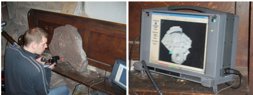
Fig. 3.3 Scanning the cross head at St John the Baptist's, Chester and a screen shot of the scanning in progress (photographs ©R.H. White)
