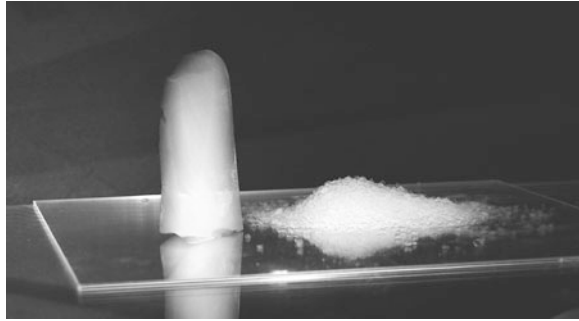
Fig. 22 Monolithic silica aerogel (on the left side ) and silica aerogel granulate ( right side )
