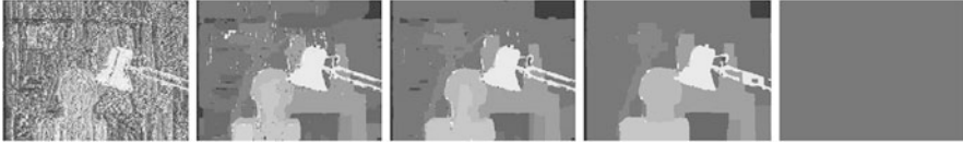
Fig. 6.8 Disparity maps for increasing values of \lambda in (6.8). The left-most image shows the result that is optimal according to the data term ( \lambda := 0 ), while the right-most image shows the disparity map optimal according to the smoothness term ( \lambda := \infty )
