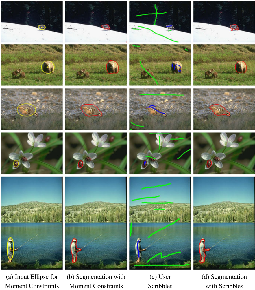
Fig. 8.11 Comparison of segmentation with moment constraints and user scribbles: Segmentation with user scribbles needs more mouse interaction to obtain similar results, since the implementation with moment constraints needs just two mouse clicks for drawing the respective ellipse
