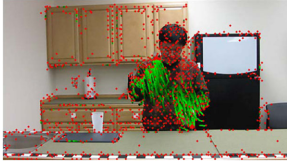
Fig. 4.1 Wang et al.’s dense features found on a sample frame from URADL’s Answer Phone activity. Red dots denote feature candidates. Green trails denote trajectory histories
