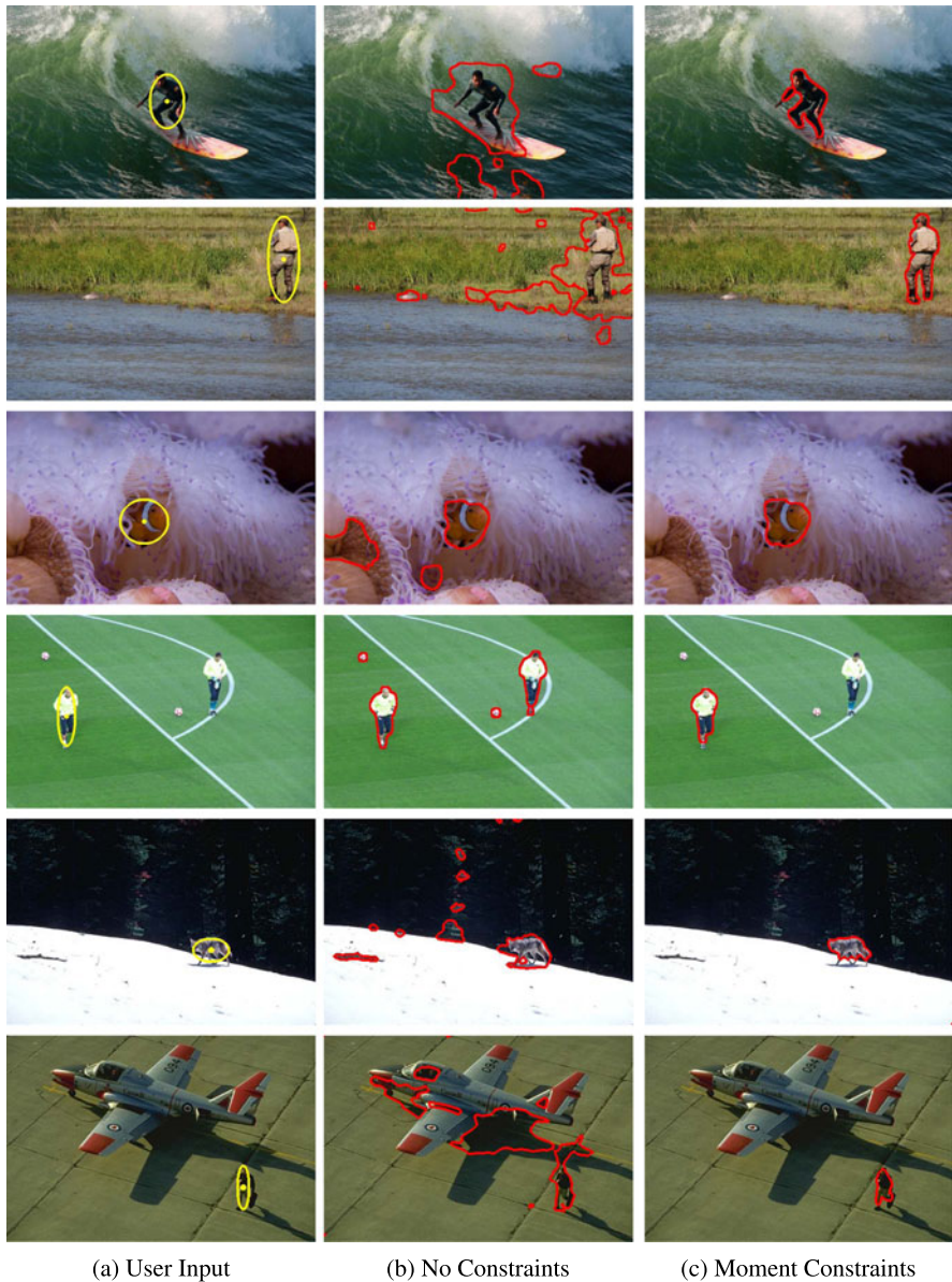
Fig. 8.8 Segmentation of real world images without and with moment constraints. (a) The user marks an ellipse at the approximate size and location of the object with two mouse clicks. Color histograms for foreground and background are determined from the inside and outside of the ellipse, respectively. (b) Segmentation results without constraints using only the histograms. (c) Segmentation results with constraints on area, centroid and covariance. Parameters of the constraints are derived from the ellipse marked by the user
