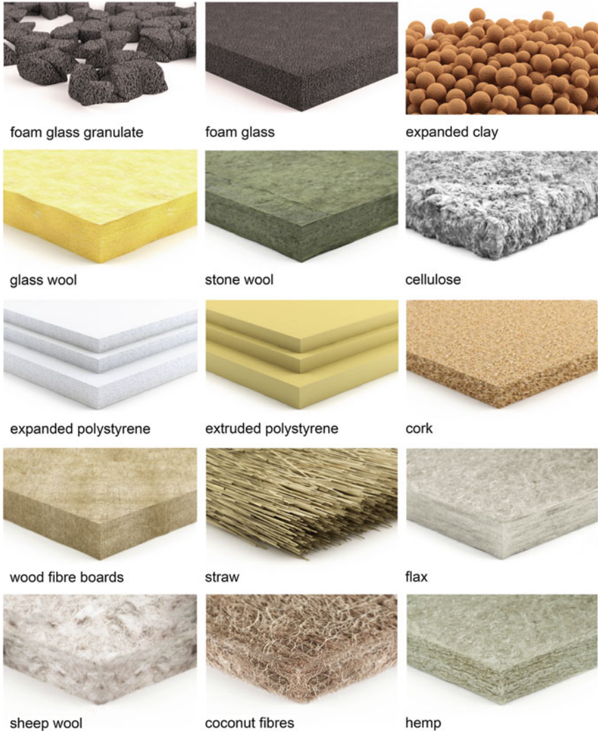
Fig. 2.12 Graphical presentation of different insulating materials
