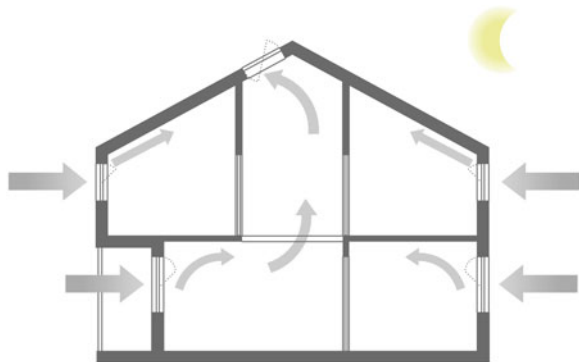
Fig. 2.23 Convective nighttime cooling by means of ventilation
