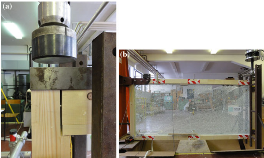
Fig. 4.39 Failure modes of the samples with a glass pane placed in the middle of the timber frame; a destruction of the timber corner in the case of using silicone and polyurethane adhesives, b a brittle glass rupture in the a case of epoxy adhesive
