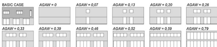
Fig. 4.13 South-oriented façade of the base—case model with the schemes of AGAW modification
