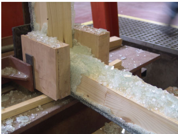
Fig. 4.36 Brittle failure mode of the glass panes in compression
