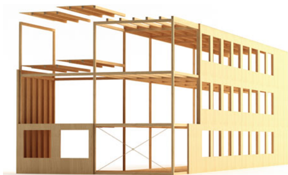
Fig. 3.30 Frame structural system—walls with an enlarged size of openings can be used in timber buildings
