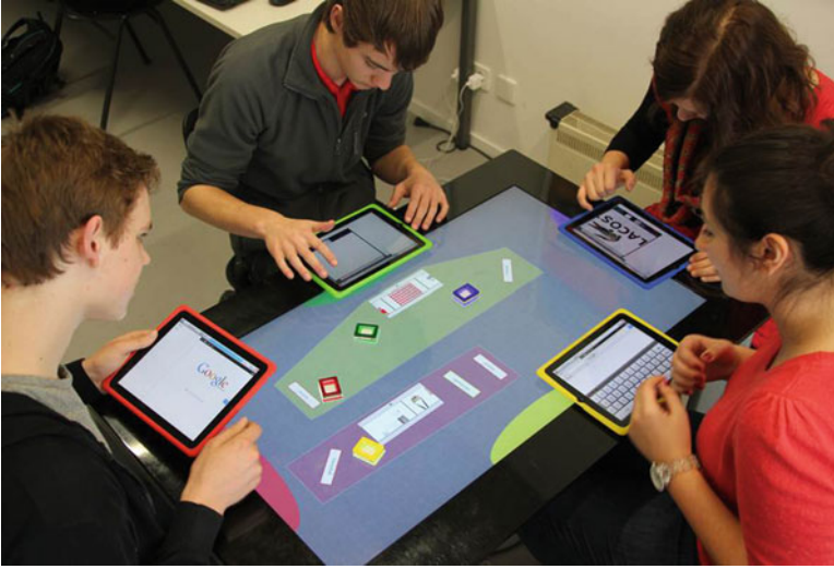
Fig. 5.1 A group of four students performing a Web search with TwisterSearch. Each student was assigned to a red , green , yellow , or blue color with which to identify themselves during the search process. The Apple iPad allows solitary Web searches as well as a seamless transition between different coupling styles without hindering others
