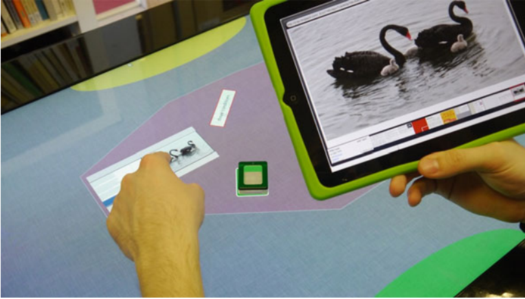
Fig. 5.6 Tapping a result in the result view on the shared display opens the same result in more detail on the private display
