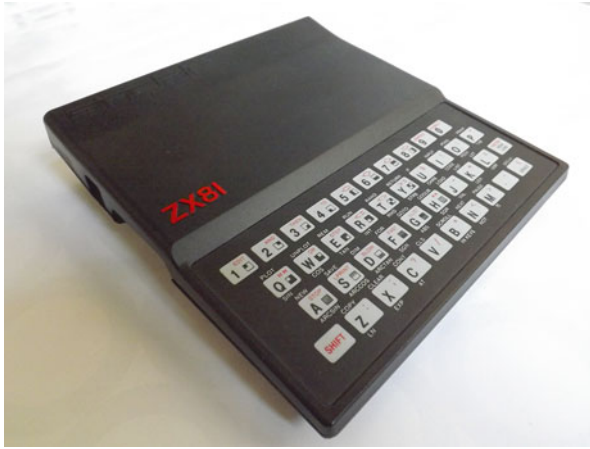
Fig. 3.1 Tinkering Users: the Sinclair ZX81. The small, flat “membrane” keyboard of the ZX81 is readily apparent, as is the minimalistic aesthetic of the machine—a simple black box ready to be plugged into a television display. The BASIC commands visible on the keys indicate the use of a keyword BASIC that allowed commands to be entered at the touch of a key. Creative users tired of the small, unresponsive keypad frequently refitted the machine with a typewriter-style unit or rehoused it in a case with a better keyboard
