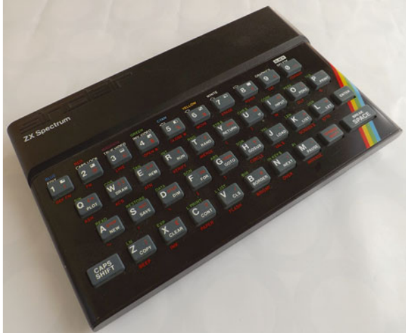
Fig. 3.2 Responding to Users: Sinclair ZX Spectrum. The larger size of the “Speccy” improved the computer’s usability compared to the ZX81 model, notably through the raised “dead flesh” rubber keys that gave computer users better tactile feedback. The machine, now with a simple sound generation and color display, was better optimized for entertainment uses than its predecessors, but BASIC programming remained a prominent part of the design
