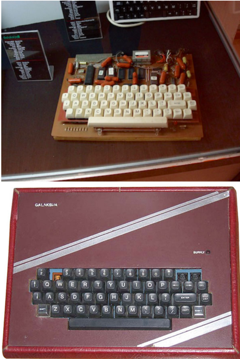
Fig. 5.3 Do-it-yourself Galaksija. Galaksija home computers were usually self-assembled by their users and did not come with a computer case. Sometimes parts were used that were compatible but not specified in the original design. While recommendations for computer case design were supplied in the original design documentation, some users chose not to use a case for the computer at all, as seen here on the image on the top . Other users customized their Galaksija cases to reflect their individual preferences, like the design shown in the image on the bottom , giving expression to their individuality through yet another medium. Of the approximately 10,000 Galaksija computers assembled, most acquired distinct looks, created by their users. Source: Courtesy Old-computers.com
