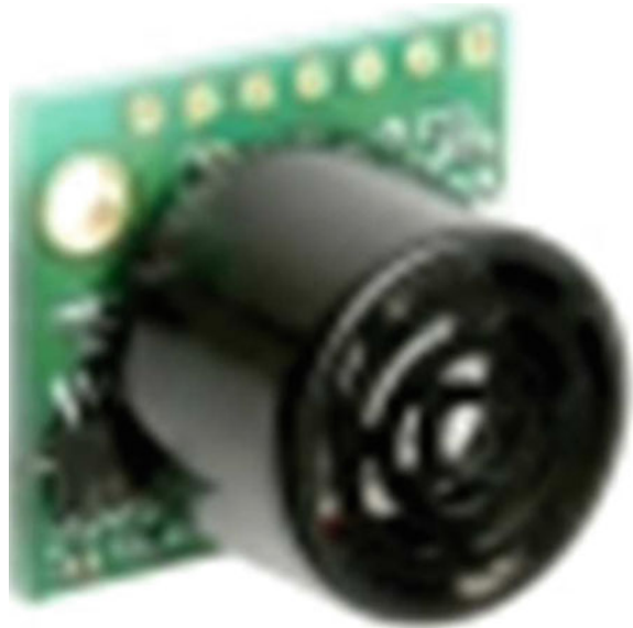
Fig. 6.7 Ultrasonic Distance Sensor Maxbotix LV-EZ1
