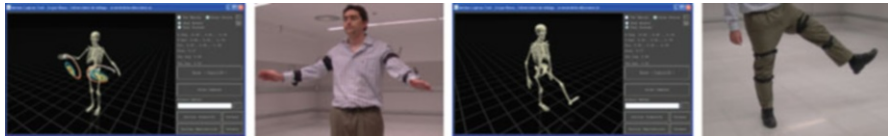
Fig. 4.8 Real-time tracking and animation of arms and legs using inertial motion capture
