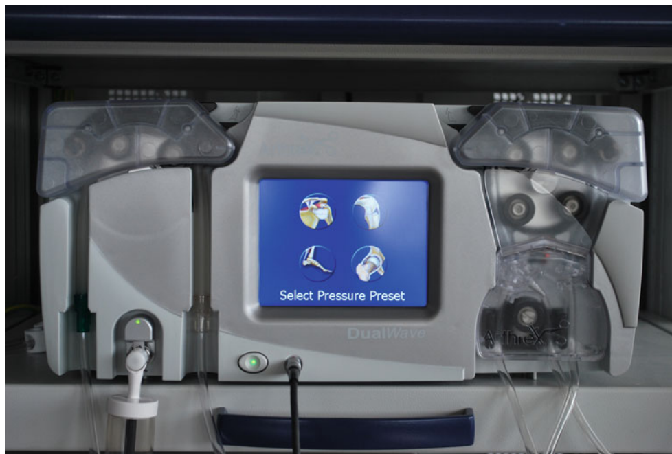
Fig. 7.2 Irrigation pump. Touch screen allows to select preset pressure and flow values according to the procedure (shoulder, knee, hip, or ankle arthroscopy) or to adjust values according surgeon's need
