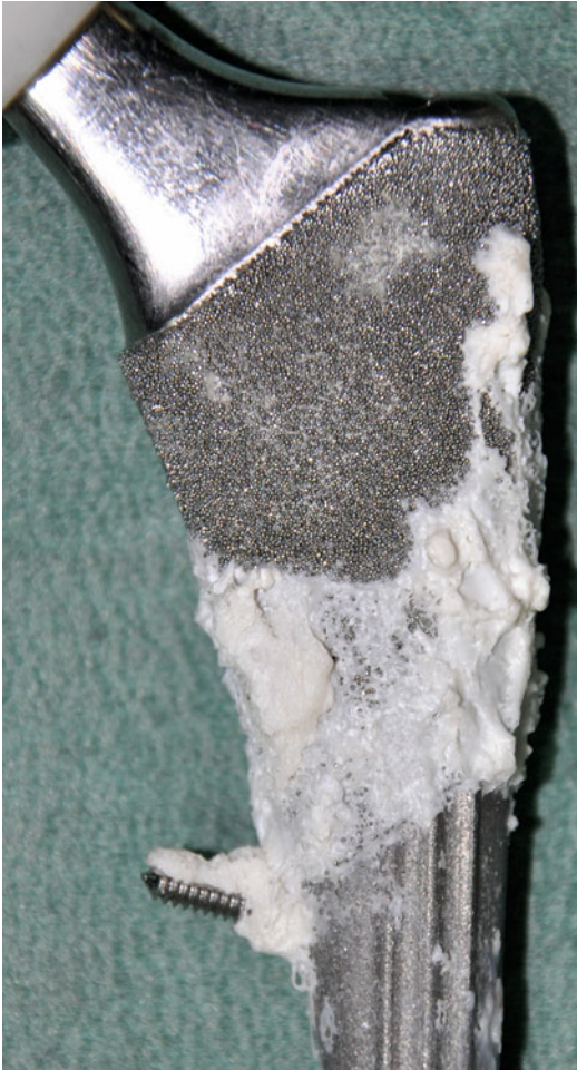
Fig. 6.1 Bone ingrowth within the porous-coated surface of a titanium femoral component
