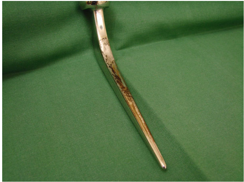
Fig. 4.1 This photograph shows an Exeter stem extracted 10 years postoperative. Note the severe crevice corrosion at the medial surface of the stem
