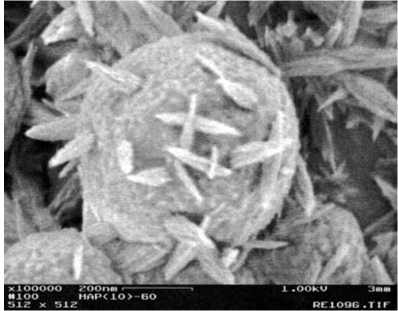
Fig. 8.2 Electrochemically deposited hydroxyapatite (BoneMaster®). Scanning electron microscope (SEM) photograph showing amorphous calcium phosphate with starting crystallization into hydroxyapatite needles on titanium (This material is reproduced with permission of John Wiley & Sons, Inc. from Rößler et al. [99])
