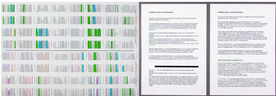
Fig. 5.4 Experiments with type to measure dot accuracy. Harman Baryta gloss fibre-based A2 with pages of type in Arial 64-up and then selecting two single pages to OCR from 64-up and 96-up, showing measurable errors. There are fewer from the 64-up page ( left ) than from the 96-up page ( right )
