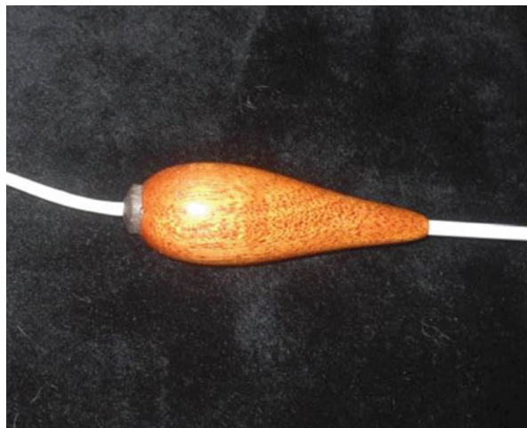
Fig. 11.1 mConduct baton containing IMU sensor
