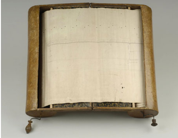
Fig. 17.5 Barbeau-Dubourg: chronographic chart 1753. The 16.5 m long scrolled timeline in its machine. The user may turn the handles to move through time. Rare Book Division, Department of Rare Books and Special Collections, Princeton University Library (Used with permission)
