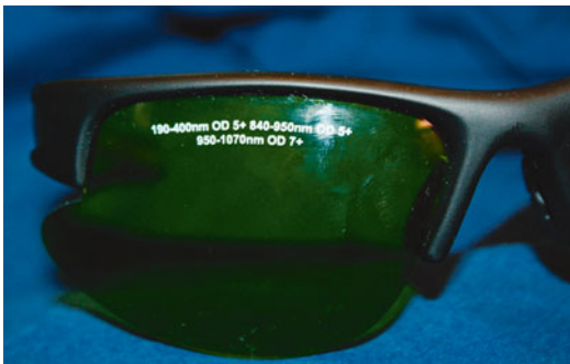
FIGURE 2.6 The optical density (OD) and wavelength are clearly marked on these Alexandrite laser goggles. This information must be permanently displayed on all protective eyewear
