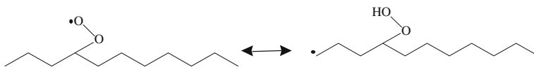
Fig. 2.10 2D-graphical form of the intramolecular abstraction of a hydrogen atom by a peroxy group presented in Fig 2.7
