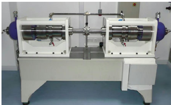
Fig. 7.4 Picture of one of the two twin-piston rapid compression machines located in the Combustion Chemistry Centre, NUI Galway
